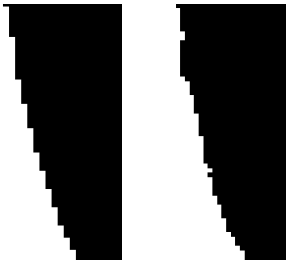
Figure 30 Optical vs Interpolated Resolution On the left is a line art edge captured using the optical resolution of the scanner (600ppi). On the right is the same edge captured using an interpolated resolution (1000ppi.) Note the greater “raggedness” of the lower quality, interpolated edge.
