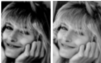
Figure 33 Maximum Density (Dmax) On the left is an image scanned with a scanner which had a Dmax of 2.5. On the right is the same image scanned with the PowerLook III, which has a Dmax, or maximum density, of 3.4. Note the much improved shadow details captured by the PowerLook III. Look specifically at the hair, and you will see how much farther along into her roots you can see.
