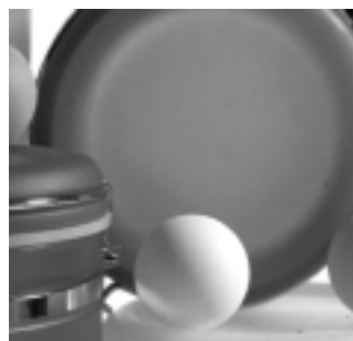
Figure 74 Newton Ring Newton ring circles can be caused by the bending and separation of light which occurs when light passes through the glass/air/image boundaries.
