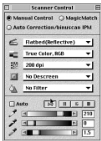
Figure 29 Scan Resolution Scanning or input resolution should be controlled through the scanning software. Scan resolutions for line art images are generally higher than for continuous tone images. Line art scan resolutions vary between 500 - 1200ppi.
