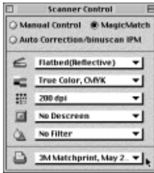
Figure 79 CMYK Conversion If you select the CMYK conversion choice option in MagicMatch, it is important to select a printer from the "Printers" menu at the bottom of the Scanner Control palette which most closely resembles your printing device. Selected here is the 3M MatchPrint proofing device, which is a common proofing device used in commercial offset printing.
