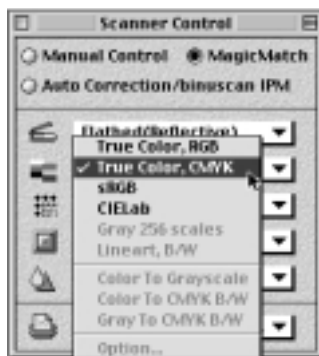
Figure 78 MagicMatch MagicMatch is selected by clicking on the MagicMatch button in the upper right hand corner of the Scanner control palette. When activated MagicMatch offers several color space conversion options not available while in Manual Control.
