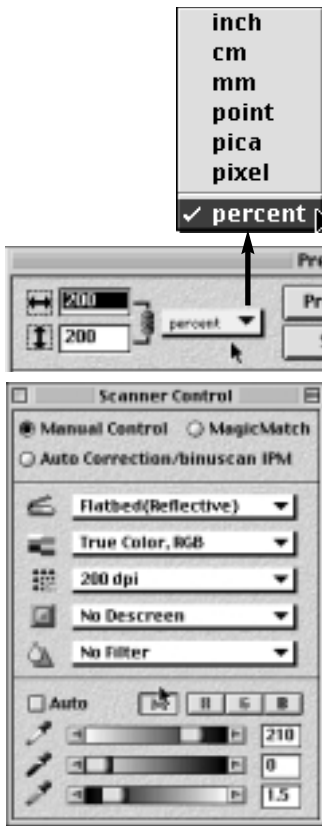
Figure 31 Scaling Setup MagicScan's scaling controls are found in the upper left-hand corner of the Preview window (top). Units can be chosen to suit your needs. Assign the final resolution you would like your image to have, here 200ppi (bottom), and the scaling which you would like the scanner to perform, here 200%. The scanner will do the rest. MagicScan will direct the scanner to scan at 400ppi, and resize the image 200%. This resizing will lower the image resolution to the requested 200ppi.
